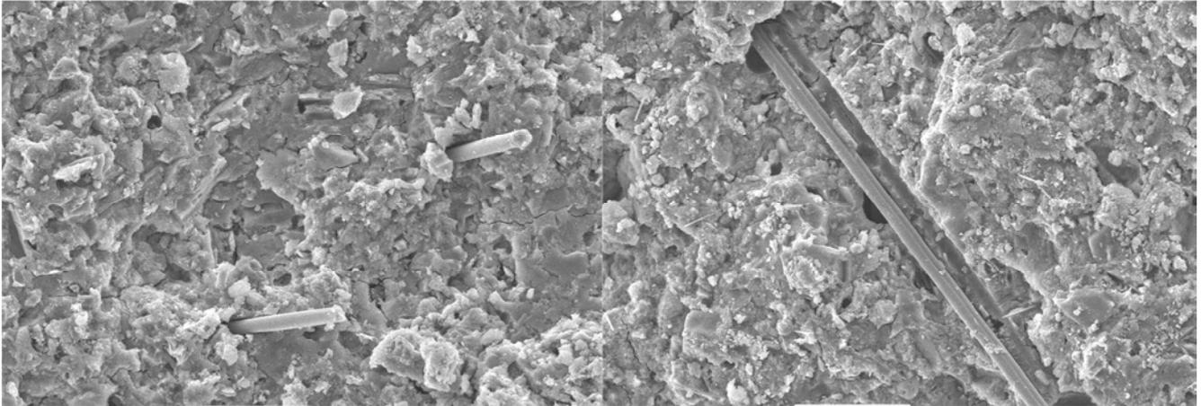
Figure 1. Fiber distribution in set cement cross section.
