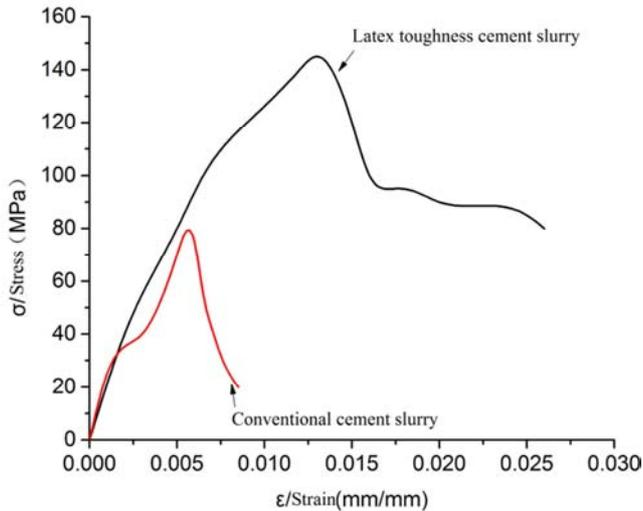
Figure 3. Set cement impact stress-strain curve.
