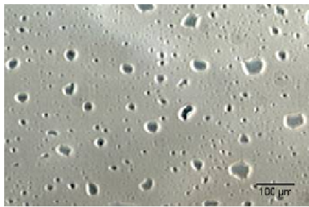
a) Initial foam (at 20 °C, P_d = 2.37 MPa)
