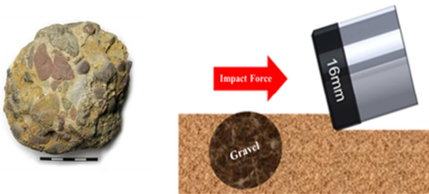
Figure 1. Conglomerate sample and the example of PDC cutter impacted by the conglomerate.
