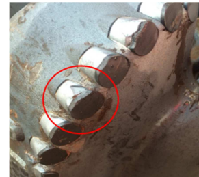
Figure 3. Conventional PDC bit cutter impact damage.
