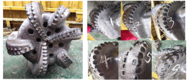
Figure 9. Bits pulled-out pictures of 17 1/2" MT616X.
