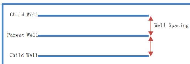
Figure 15. Infill wells are completed 6 or 60 months after parent well.
